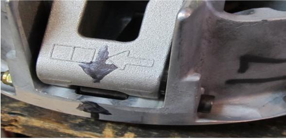
After removing the outer clutch assembly from the vehicle, mark the moveable sheave and governor assembly for location for re-installing later.
