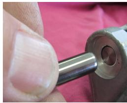
The pin tool will temporarily hold the 3 parts in place until you press the axle pin into the spider.
