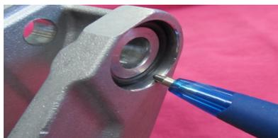
On some models (like some Skidoo 1200cc 4 stroke) there is a rubber compression o-ring under the plastic slider shoe, be sure to keep track of it for re-installing later.
