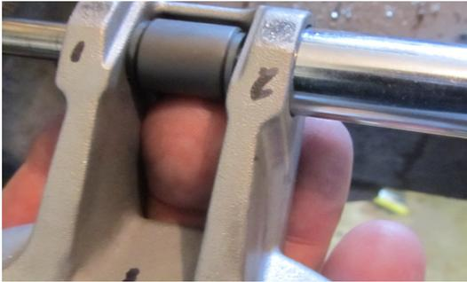
**Watch closely as the axle goes through the vespel washers,** you may need to slightly move / guide the washers with a probe.
